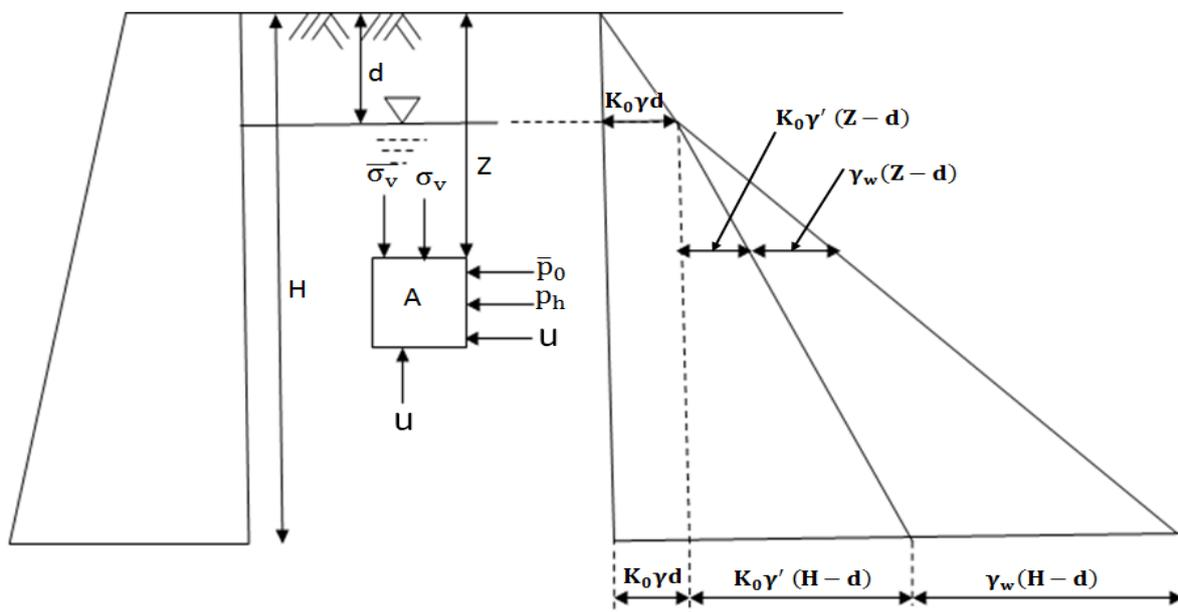
The vertical stress ' $\sigma_v$ ' at depth 'd' above the ground water table from the top is given by
