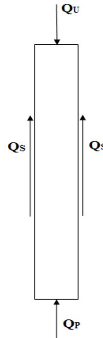
The pile load test is most reliable method to determine the ultimate load capacity of a pile. In pile load test, the test pile is driven and loaded up to failure.
