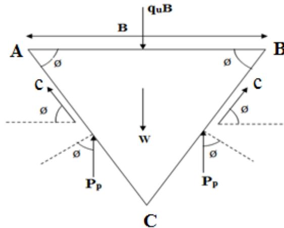
The resultant passive earth pressure ( $P_p$ ) will acts vertically upward making an angle ' $\phi$ ' with the normal to the surfaces 'AC' and 'BC'.
