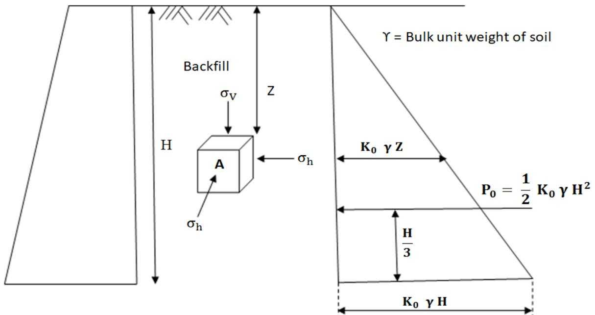
But in 'At-Rest Earth pressure' condition, the retained soil or backfill is not subjected to any lateral movement and hence the lateral strain ' $\epsilon_h$ ' of the soil element in the horizontal direction is equal to zero.
