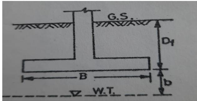
**Case 01 :** If  $b \geq B$  then there is no change in the Terzaghi's bearing capacity equation
