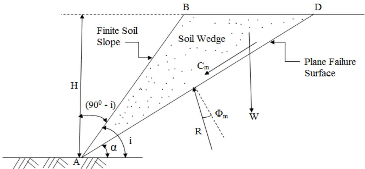
Let us consider the equilibrium of the triangular soil wedge 'ABD' formed by the inclined soil slope surface 'AB' and the assumed plane failure surface 'AD' as shown in figure.
