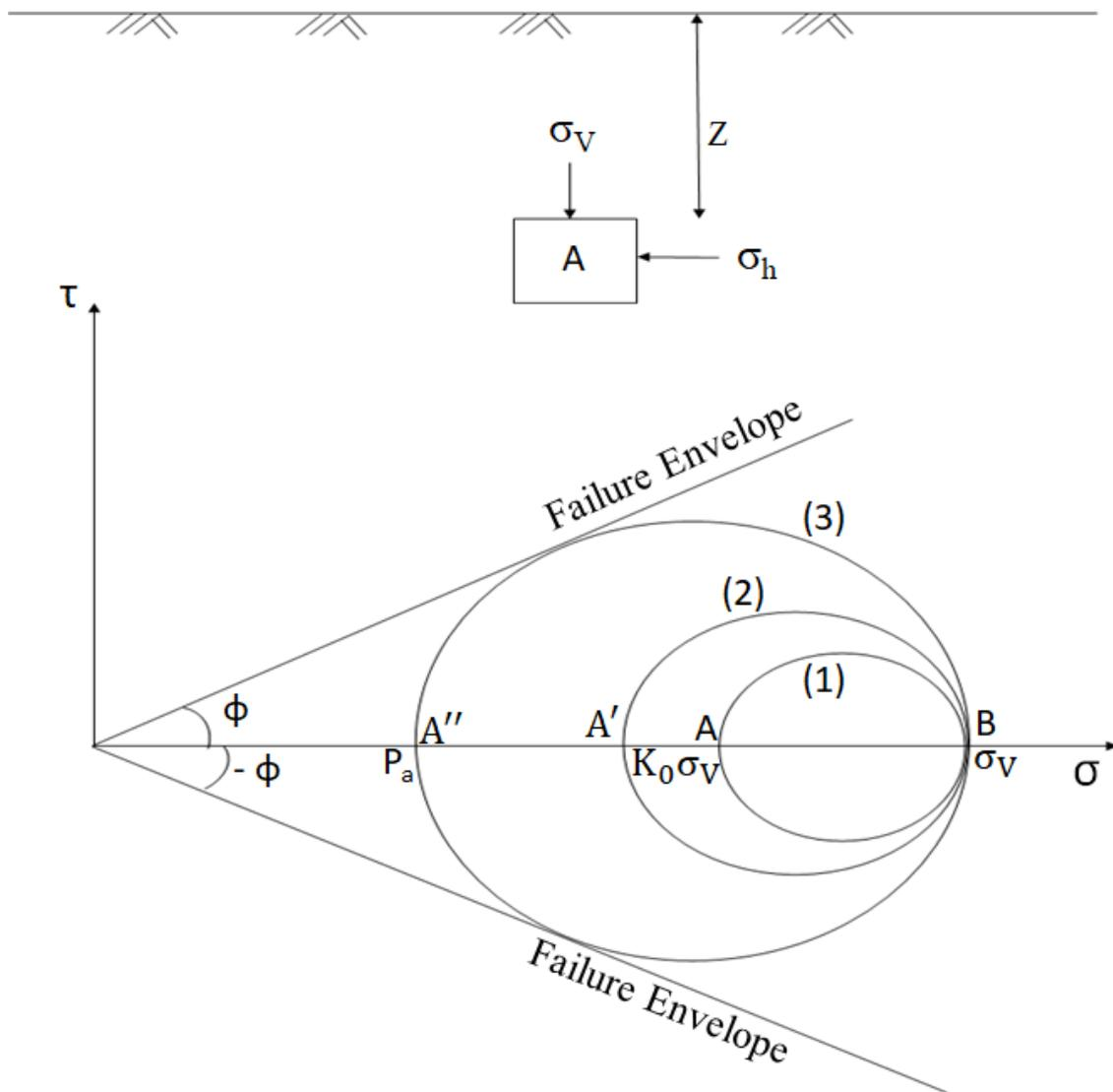
Thus, at this limiting minimum condition of horizontal principal stress, the soil is at the verge of shear failure and it has said to attained the Rankine’s active state of plastic equilibrium.
