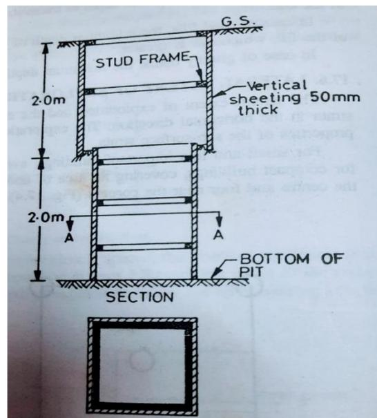
Shallow pits up to a depth of 3 m can be made without providing any lateral support. For deeper pits, especially below the ground water table, lateral support in the form of sheeting and bracing system is required.
