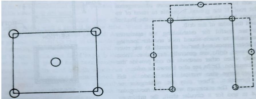
For highways, subsurface explorations are usually carried out along the proposed centre line (or) along the proposed ditch line. The spacing of bore holes usually varies between 150 m to 300 m. If the sub-strata is erratic, the spacing may be reduced to even 30 m.
