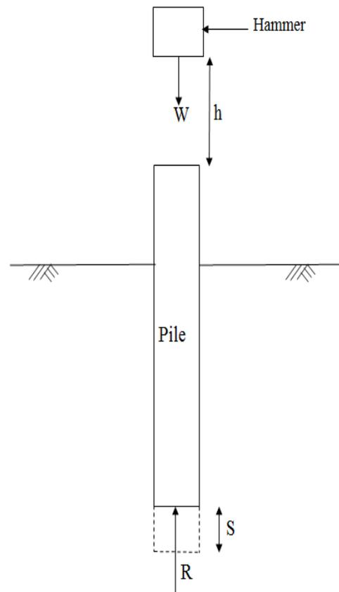
The following dynamic formulae are used in pile foundations
