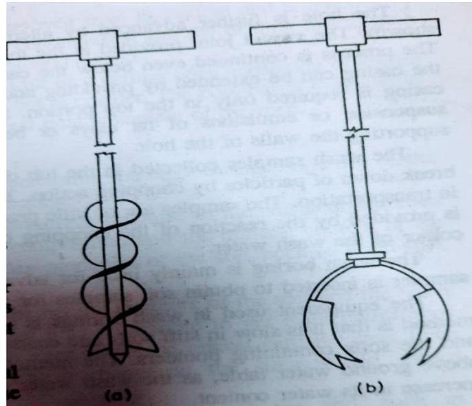
The hand augers used in boring are about 15 to 20 cm in diameter. These are suitable for advancing bore holes upto a depth of 3 to 6 m in soft soils.
