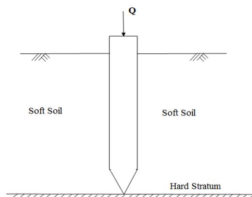
The friction piles are used when the hard stratum does not exist at a reasonable depth from the ground surface.
