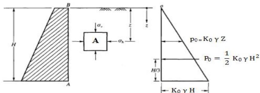
The earth pressure ( $p_0$ ) at the bottom of retaining wall at depth 'H' is given by
