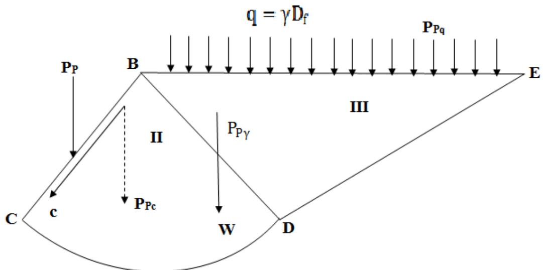
The resultant passive earth pressure ( $P_p$ ) acting in Zone – II and Zone – III has the following three components
