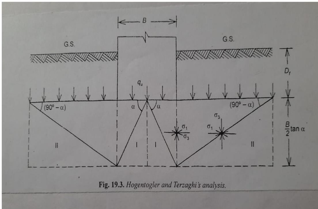
At the time of failure, the foundation exerts a pressure “ $q_u$ ” equal to the ultimate bearing capacity of the foundation soil.
