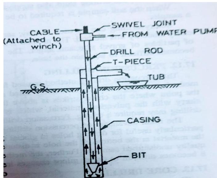
The water emerges as a strong jet through a small opening of the chopping bit. The hole is advanced by a combination of chopping action and the jetting action, as the drilling bit and the accompanying water jet disintegrate the soil.
