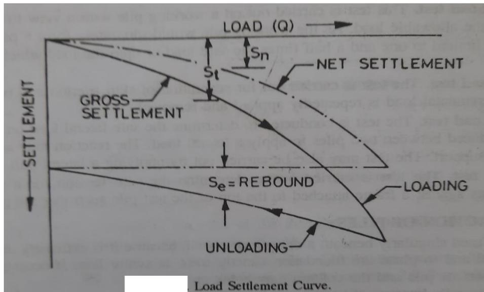
The figure shows the load – settlement curve for loading as well as for unloading obtained from the pile load test.
