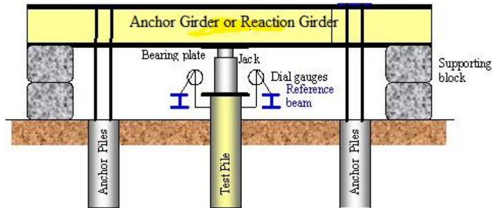
The pile load test is the most reliable field test for determining the load carrying capacity of a pile. The pile load test set-up generally consists of two anchor piles supporting an anchor girder or a reaction at their top as shown in the figure.
