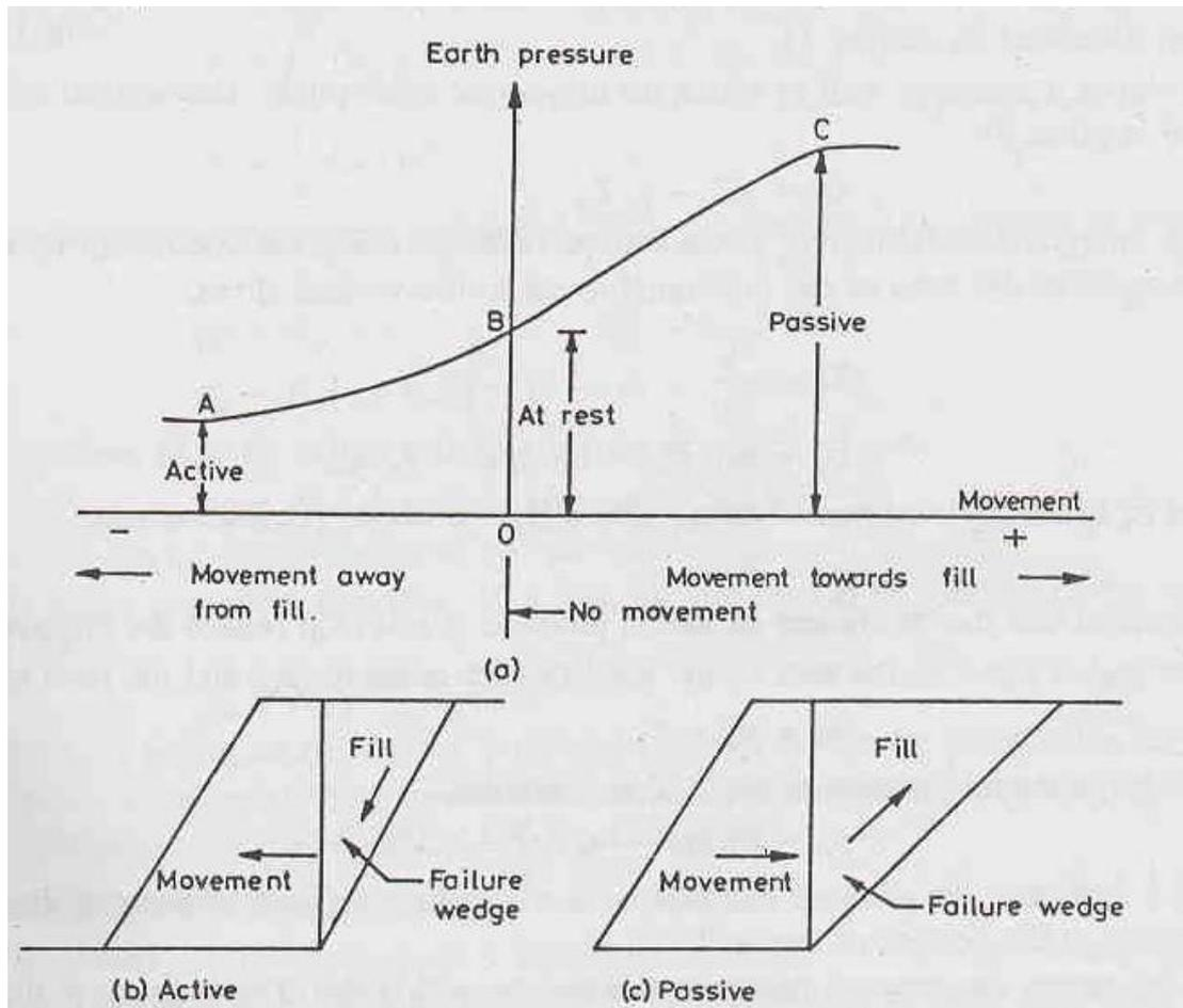
The point 'A' in the figure indicates the case when the retaining wall moves away from the backfill. It indicates the state of 'Active earth pressure'.
