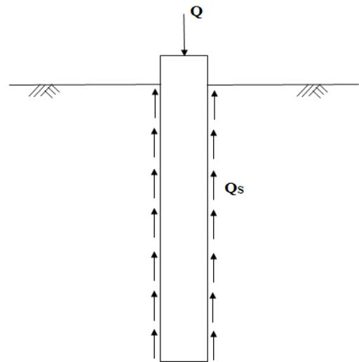
The combined end bearing and friction piles transfer the loads by a combination of end bearing at the bottom of the pile and friction along the surface of the pile shaft.
