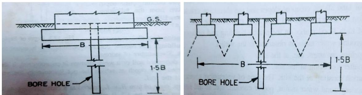
In the case of pile foundation, the depth of exploration below the tip of bearing piles is kept at least 1.5 times the width of the pile group.
