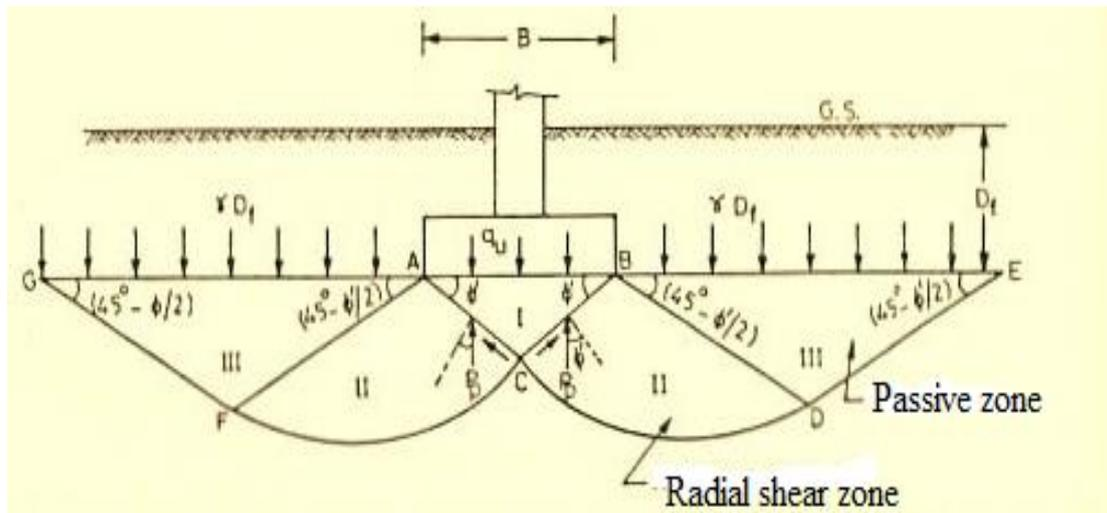
The region in the failure surface "GFCDE" is separated into five zones
