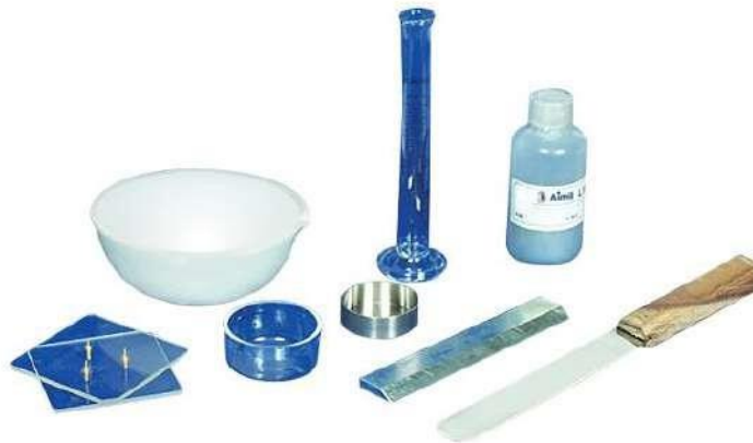
Apparatus required for Shrinkage Limit test
