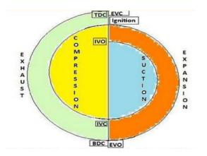
But actual valve timing diagram is different from theoretical due to two factors-mechanical and dynamic factors. Figure 4 shows the actual valve timing diagram for four stroke low speed or high speed engine.
